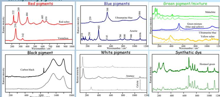
Fig. 3. Raman spectra of pigments used in the wall painting. Dotted lines - reference Raman spectra.
