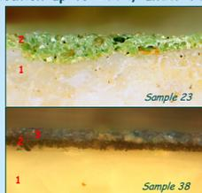
Fig. 2. Microphotography images of cross sectioned samples: Sample 23/ green color and Sample 38/ blue color. Legend: 1- ground; 2, 3- pictorial layer.
